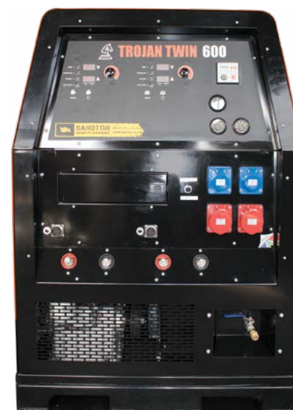
All the welding controls and the digital displays are placed on the front panel of the multipack, with plug-in connections to the power sources made via power cables and harnesses.
